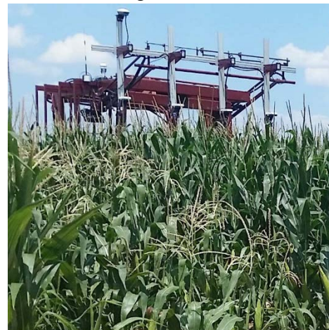
Figure 2: Ground based phenotyping machine that can measure mature corn without damage. The first of its kind in the world and is expected to save labor
